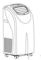
Drainage Hole Rubber Plug
